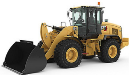
Caterpillar 938 Front-End Loader
